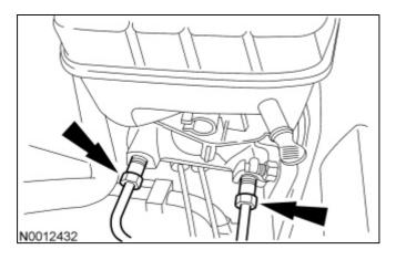
2. Install short brake tubes onto the primary and secondary ports with the ends submerged in the brake master cylinder reservoir.
