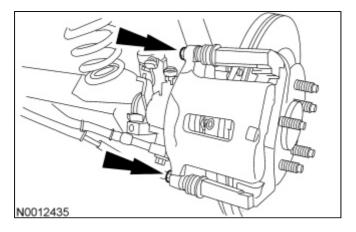
7. Remove the brake caliper bleeder screw cap and place a box-end wrench on the bleeder screw. Attach a rubber drain hose to the bleeder screw and submerge the free end of the hose in a container partially filled with clean, specified brake fluid.
