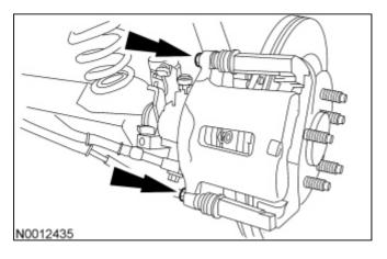
3. Remove the outer brake pad.
