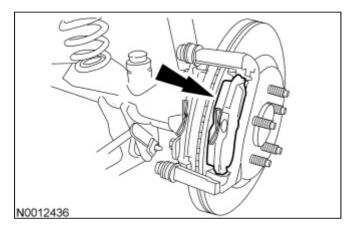
4. NOTE: Place a shop towel between the caliper and the brake disc.
